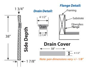
FEATURES Dimensional Tolerance ± 1/8". Dimensions needed for site preparation should be measured from the unit. American Bath Group assumes no responsibility for preparatory work.
