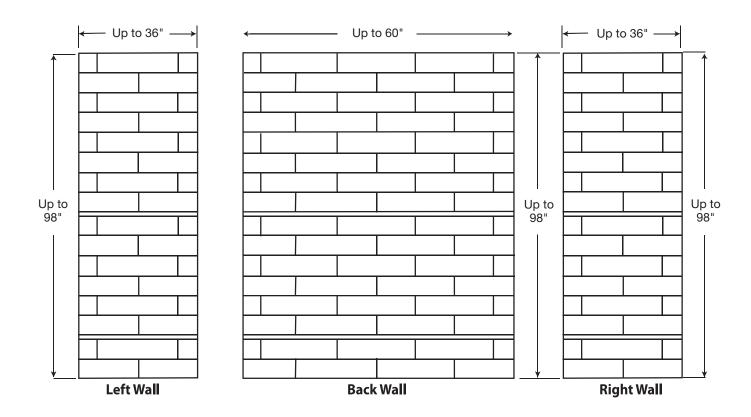
$\textbf{FEATURES} \ \ \text{Dimensional Tolerance} \ \pm \ \textbf{1/6}". \ \ \text{Dimensions needed for site preparation should be measured from the unit. American Bath Group assumes no responsibility for preparatory work.$
