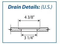
FEATURES Dimensional Tolerance ± 1/8". Dimensions needed for site preparation should be measured from the unit. American Bath Group assumes no responsibility for preparatory work.
