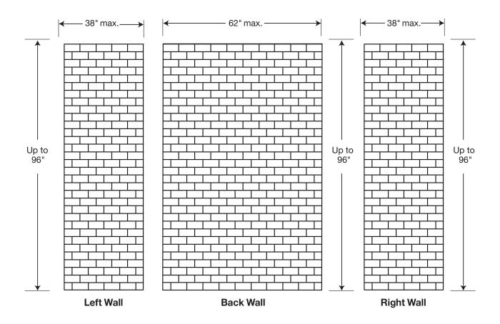
FEATURES Dimensional Tolerance ± 1/6". Dimensions needed for site preparation should be measured from the unit. American Bath Group assumes no responsibility for preparatory work.
